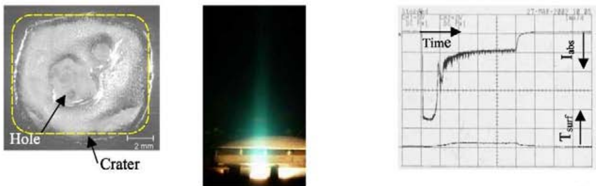
Fig. 44 Surface morphology, digital camera, absorbed current of stainless steel (M139_75) P_{\text{abs}} = 1.6 \text{ GWm}^{-2} \Delta t = 5 \text{ ms} (loaded in JUDITH)
